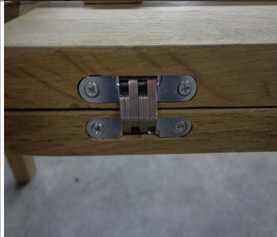
Soss hinge to allow the inlays to fold.
