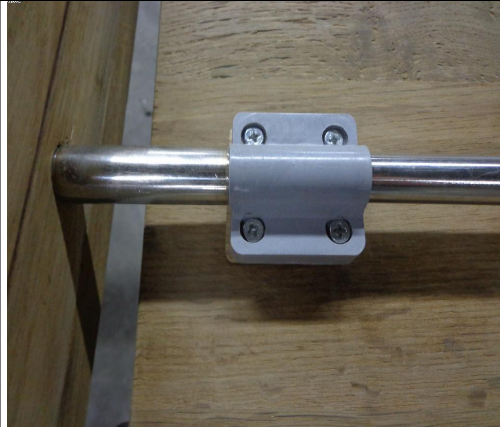
Plastic Block for correct height of inlay.
