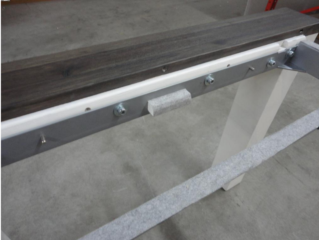
Stopper and frame for storage of inlay. Its covered with felt to avoid damage.
