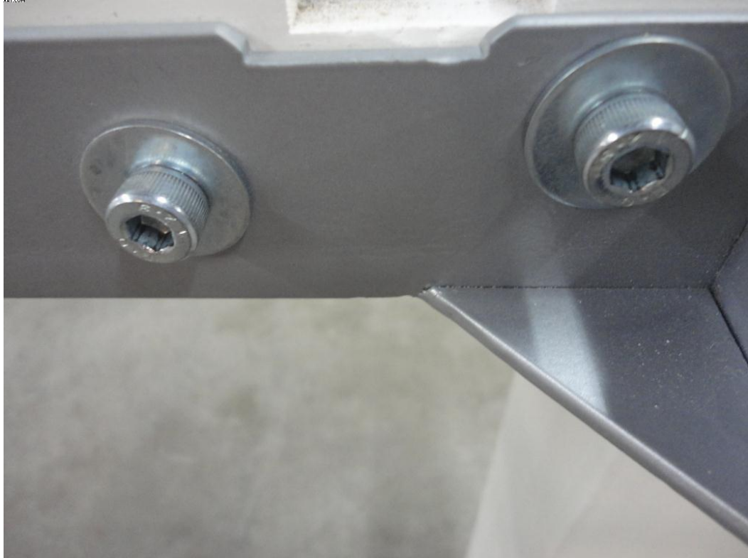
Bolts for fixing frame to movable leg.
